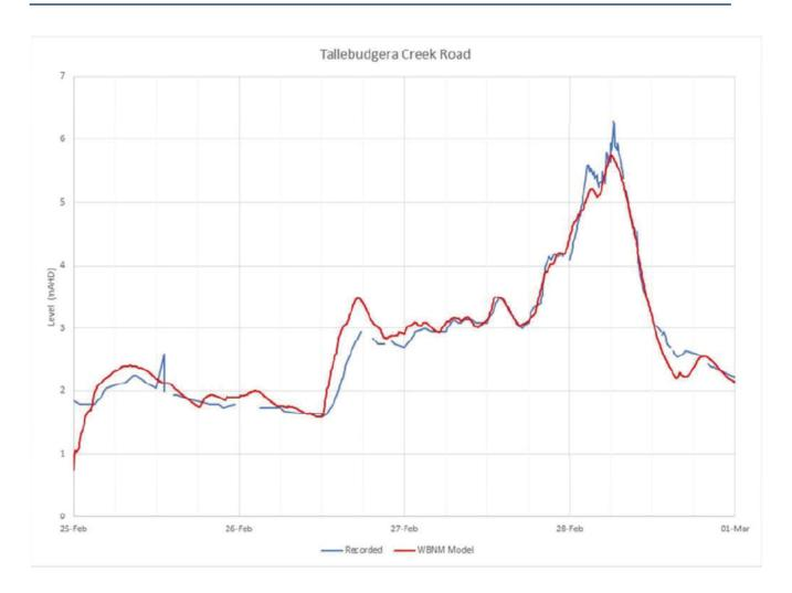
32 These results are consistently good. The modelled results closely mimic the recorded levels, providing a high level of confidence that the WBNM hydrologic model is accurately transforming actual rainfalls into measured flow rates.
