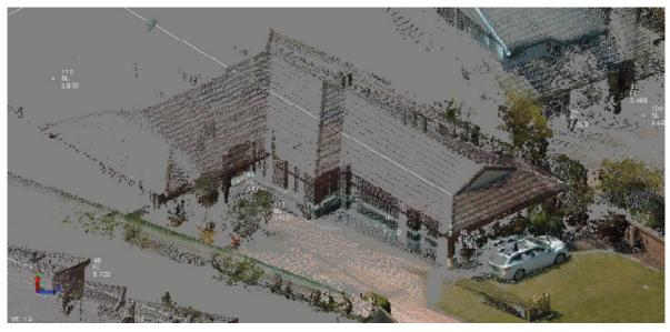
Figure 2 – Example point cloud
